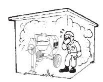
narrow area where free flow of the air is restricted. If the air flow is restricted it will cause serious damage to the mixer or engine and may cause injury to people and property. Remember the mixer's engine (gasoline models only) gives off **DEADLY** gases.
